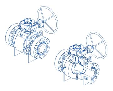
Our flexibility towards delivering an optimised surface Ball Valve solution ensures that both client and governing industry requirements are always met, and allows for a fit for purpose final product to be delivered on time and within budget. Additionally the E-Ball Valve is a patented product that provides double block and bleed (DBB) functionality within a single valve.
