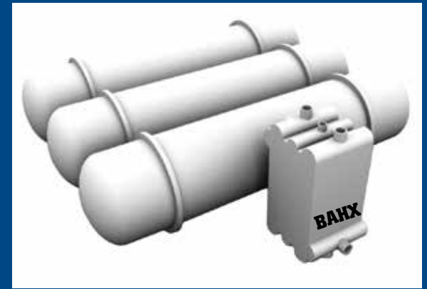
BAHX footprint comparison vs. shell and tube technology
