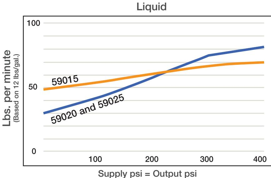
Actual flow rates will depend on the liquid or vapor phase of the refrigerant, the inlet pressure and outlet pressure required
