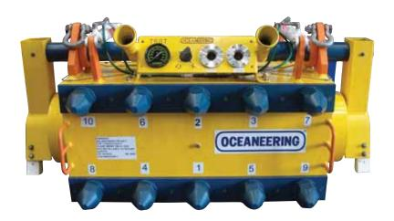
The Diverless Smart Clamp is a split mechanical / hydraulic fitting used to repair a damaged or leaking subsea pipeline. The fitting eliminates costly pipeline shut downs and offers an alternative to hyperbaric welding repair methods.
