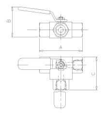
The 'B6SL' Type 3 way Flow Diverting Ball Valve is designed for safely diverting flow to one of the two outlet ports. Totally enclosed soft seats offer both positive sealing and low operating torques, from vacuum to high-pressure service. Anti-blow out spindle is fitted as standard with the PTFE spindle and body seals.
