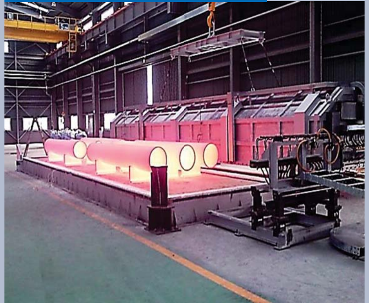
Heat Treatment Furnace for Seamless Pipe
