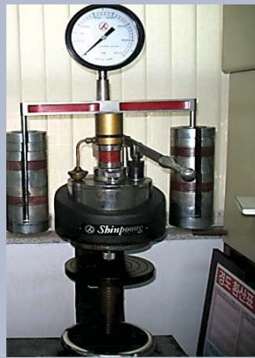
BRINELL HARDNESS TESTER(305HB)
