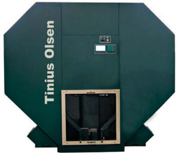
Impact Test ( - 196°C )
