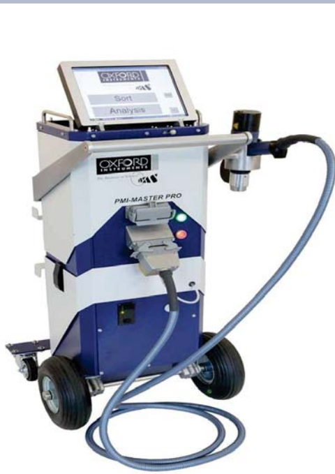
PMI Master Pro(SS, DSS, AS, Non-Ferrous)
